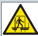
Danger Fragile roof
