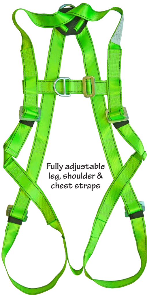
Rear dorsal plate slides upwards to keep the user upright after a fall
