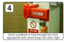
Please note that the holes on the slider have a staggered repeat which ensures that at least one hole will be tight when placed against the valve. If more than one padlock is required then a hasp should be used on the hole which keeps the slider as tight to the valve as possible.
