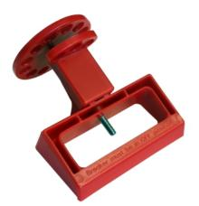
Designed for 3 phase breakers, this large lockout fits over the switch and then the screw is tightened using the clock style section. When tight the clock section is locked to the main body through a sliding section fitted to the main body.
