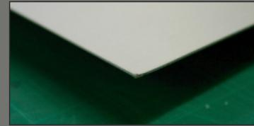
Zintec is a steel sheet that has been electro-coated with zinc. This coating protects the sign from corrosion.
