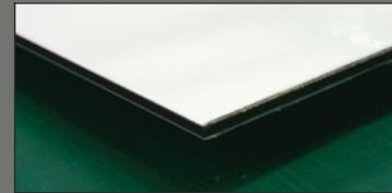
Dibond is an aluminum composite material made of two lightweight sheets of aluminum with a solid black thermo-plastic core.
