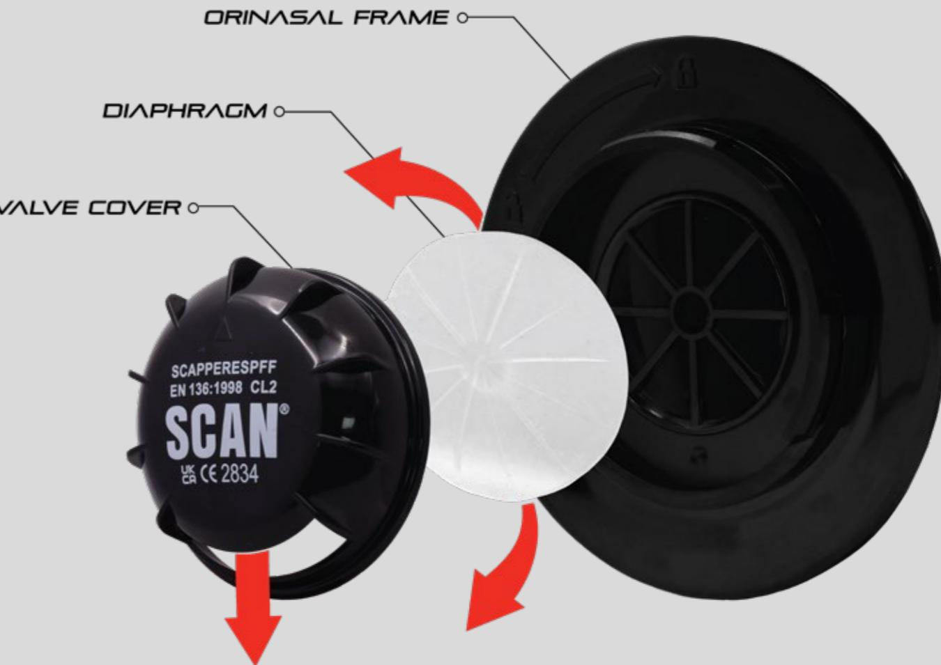
When the diaphragm opens, exhaled air that would otherwise become trapped beneath the upper section of the valve cover and hinder further exhalation can flow out through the vents, ensuring exceptionally low breathing resistance. The diaphragm is made from silicone, which resists moisture and maintains its high performance even in very low temperatures.
