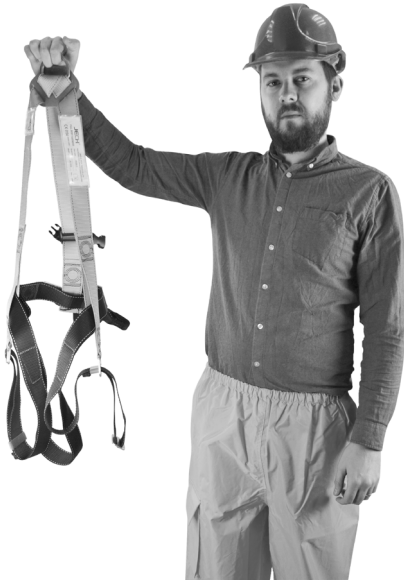
A) Open the leg loop buckles and, holding the shoulder straps, put on the harness like a vest.
